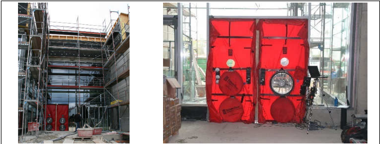
Figure 30: Airtightness measurement: the fan built-in. For the measurement of airtightness only one fan needed
