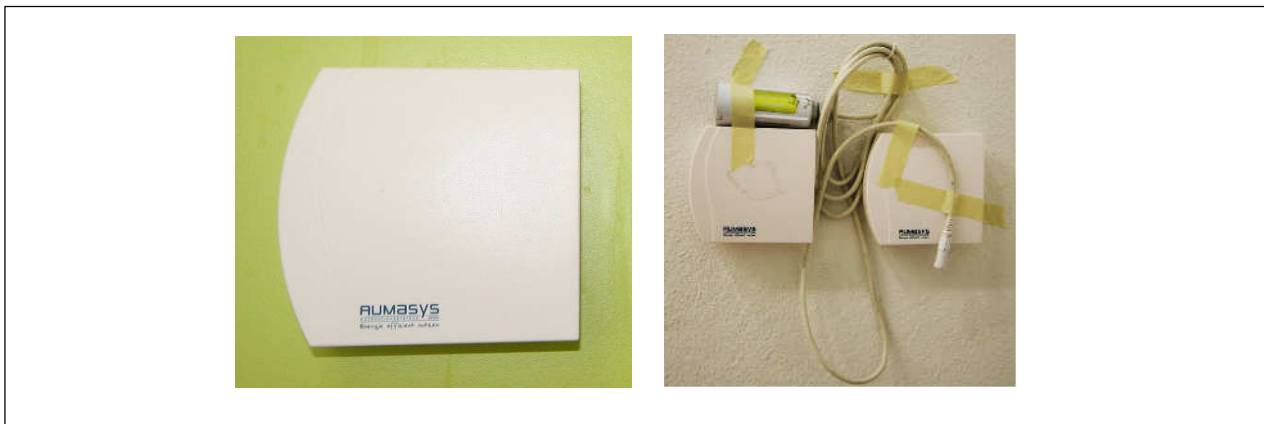
Figure 8: left: wall sensor For temperature and relative humidity, right: wall sensor with data logger for calibration (temporary)
