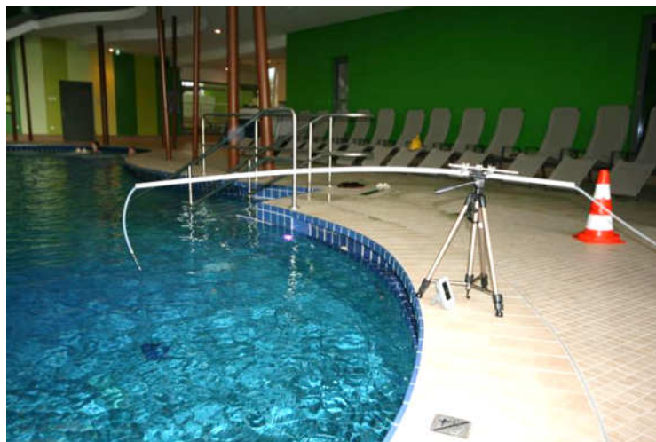
Figure 62: Measurement of trihalomethanes 20 cm Leisure pool, air intake on activated carbon
